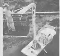
LAGO'S NEW Pitman Giraffe can quickly and safely put a tank painter high in the air. He controls his movement from the platform. E PITMAN Giraffe nobo di Lago por pone un verfo di tank liher y siguramente den aire. El ta controla su movimiento for di e plataforma.
